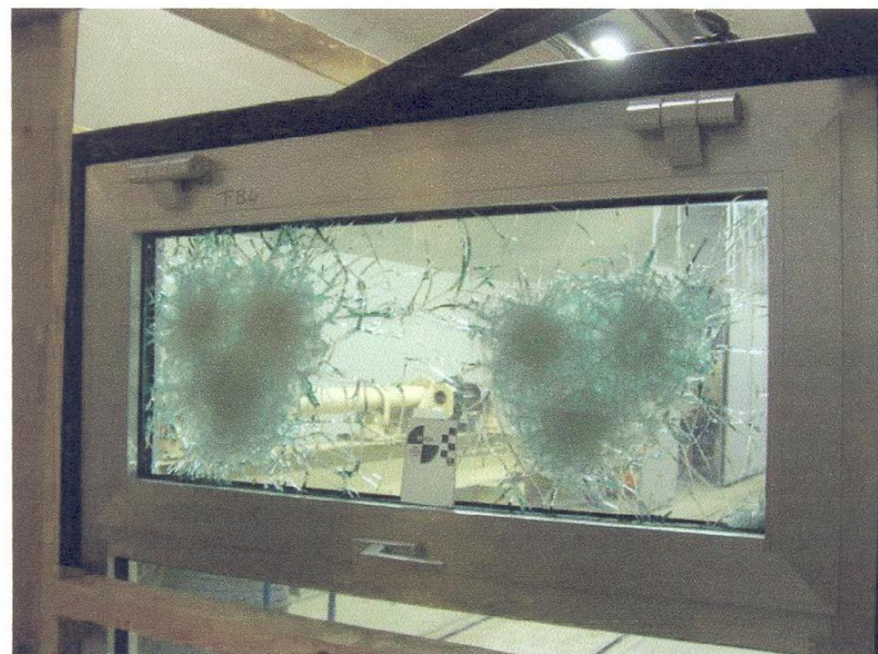
Figure 2 : Back sample AR 83 - FB4 after testing with .357 CB and .44 FMJ.
