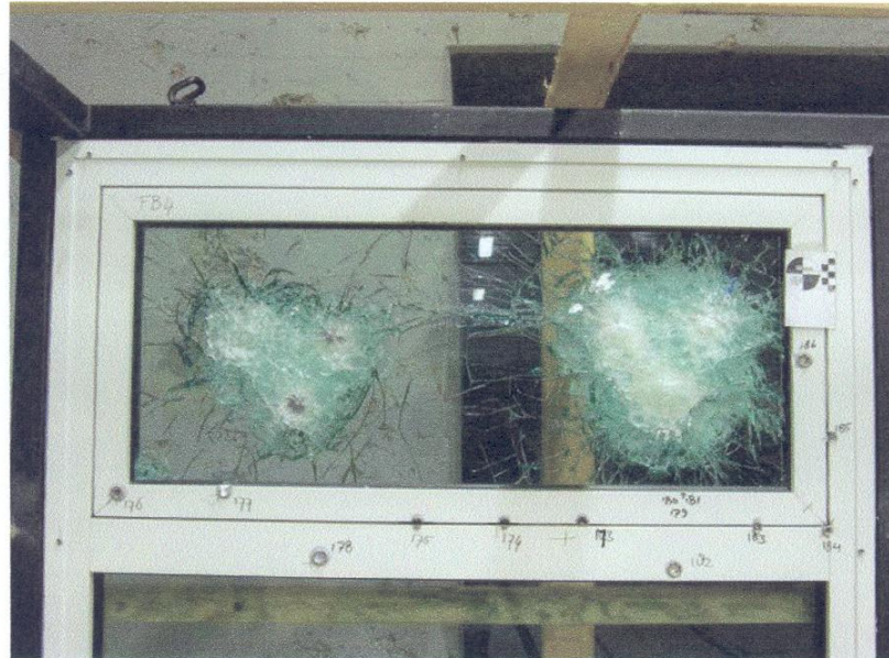
Figure 1 : Front sample AR 83 - FB4 after testing with .357 CB and .44 FMJ. Shot no. 05SN182 until 189 concerning .357 CB.
