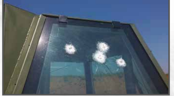
7,62x51 AP testi 7,62x51 AP testing
